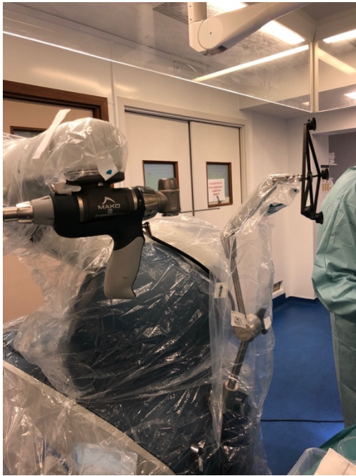
(b) A MAKO Haptic hand-held saw for UKR
